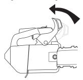
Unscrew the bar nut and remove the clutch cover (chain brake). Take off the transportation ring (A).
